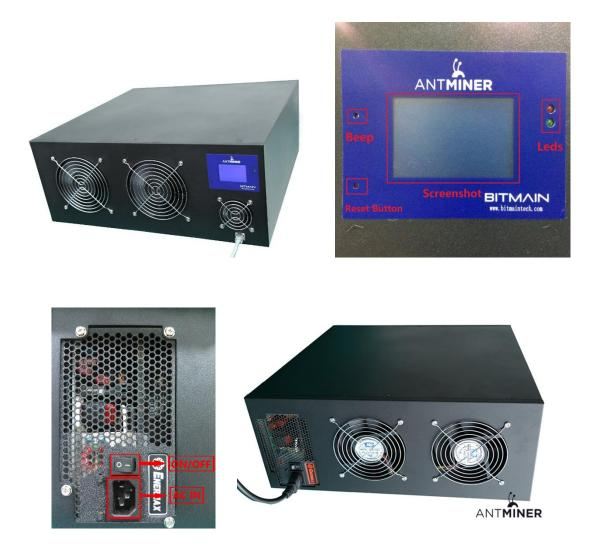
1000W PSU: when you set up S2 server, only need to connect to AC 220V/50Hz or 110V/60Hz. LCD screen: here show IP Address, Hashrate, the highest temperature. There are also Status LEDS, Reset button and Beeper on the screen.
